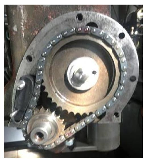
A quite simple and useful timing chain tensioner modification to a side valve USHM 918cc. It could be done on a UB engine too and is something to consider if you run at 4000 RPM a lot.
