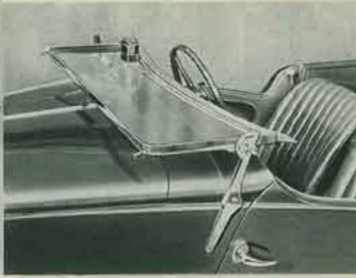
On the open models the adjustable windscreen can be folded right down on to the scuttle when required thus providing clear vision in fog or frosty weather.
