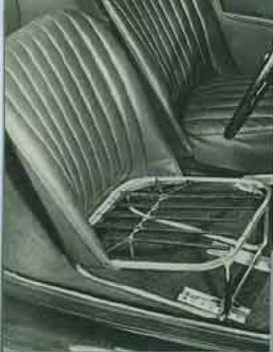
The seats on all models are of the metal framed easy-chair type with floating spring base and comfortable upholstery.
