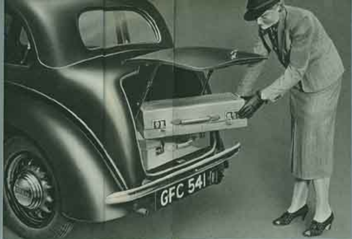
On the Saloon models the large built-in luggage container has external access by hinged lid with door-type lock. The capacity of the container is nearly 5½ cubic feet.
