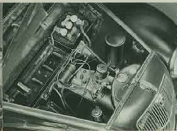
The power unit has been considerably improved by the provision of a balanced crankshaft, tin-coated aluminium pistons, improved manifold and improved lubrication. All maintenance adjustments are easily accessible.
