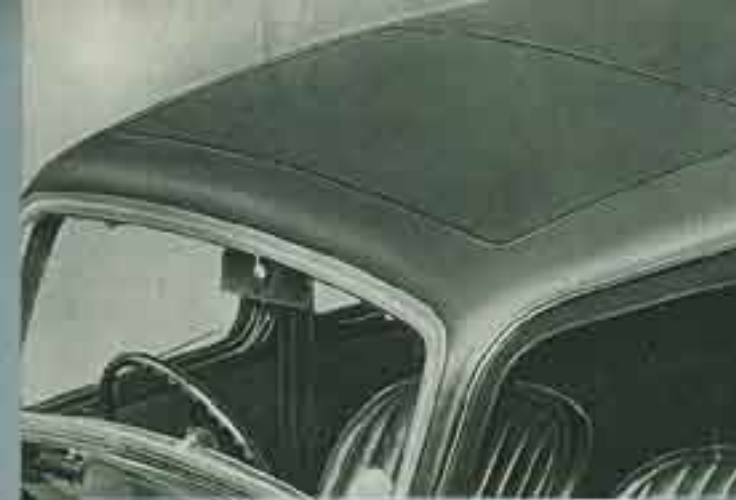
The sliding head is of the flush fitting type and provided with concealed drainage ducts which discharge all rain water below the car.
