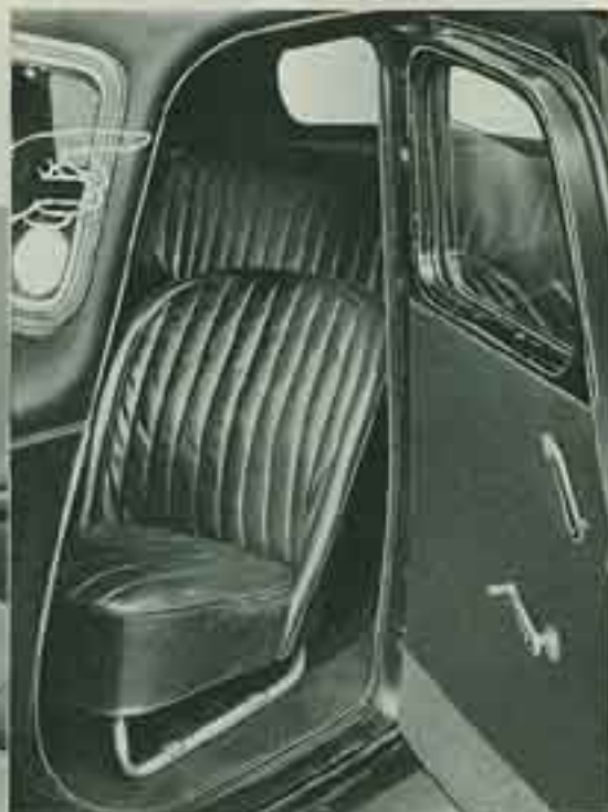
Special care has been taken to render the new Morris Eight weatherproof. Note the way the roof guttering is carried right down below the door to discharge water on to the road.
