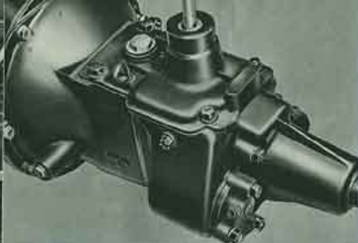
The new four-speed gearbox has silent helical gears and synchromesh engagement on second, third and top gears. In addition the driven shaft is supported on three bearings.
