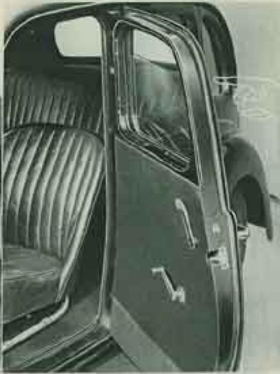
Objectionable draughts are guarded against by rubber draught welts round the doors of the Saloon models. Similar care has been taken at other points of the body.
