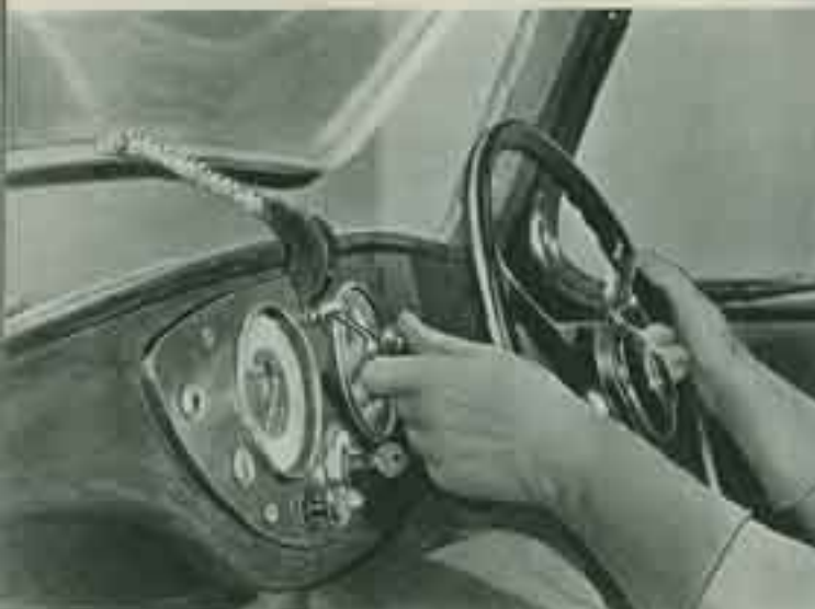
On the Saloon models the instruments are attractively grouped high on the fascia board to facilitate easy reference. The opening windscreen is controllable to a wide angle by the central winding regulator.
