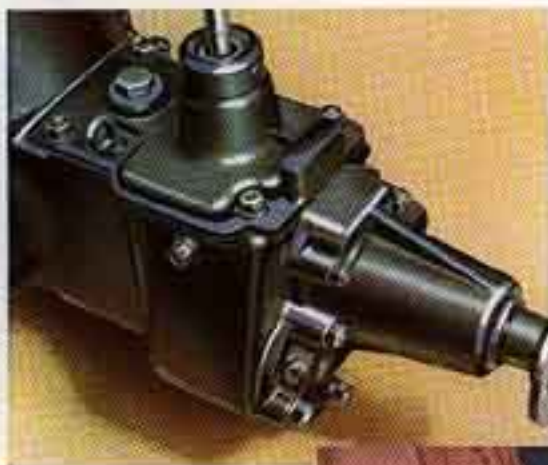
The new four-speed gearbox has synchromesh engagement for 2nd, 3rd and top gears, and is provided with silent helical gears.
