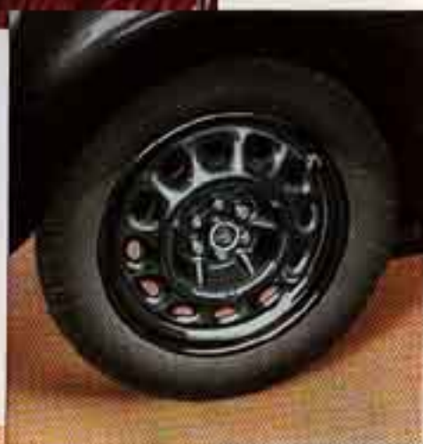
Improved spoked-disc easyclean wheels with six-stud fixing and large tyres are fitted.
