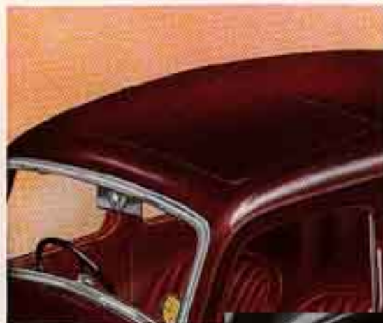
The sliding head saloon models are fitted with a flush fitting sliding head with concealed guttering discharging water below the car.
