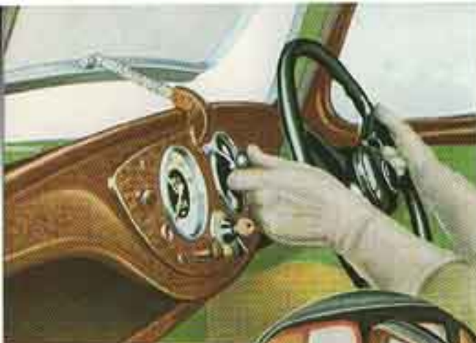
The windscreen has central winding control and opens to a wide angle.
