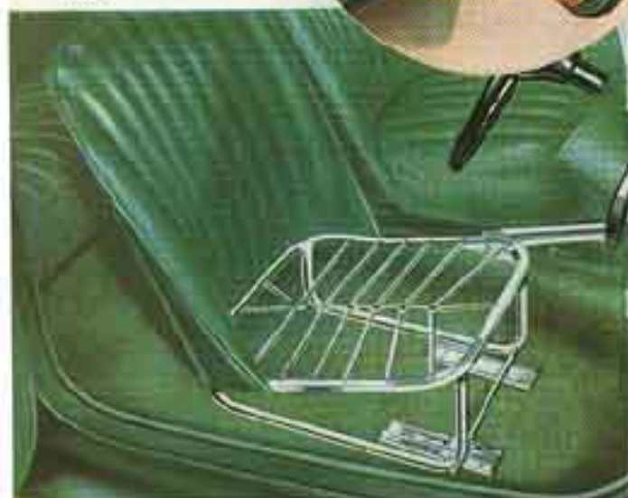
The front seats are of the metal framed easy-chair type with floating spring seat base.
