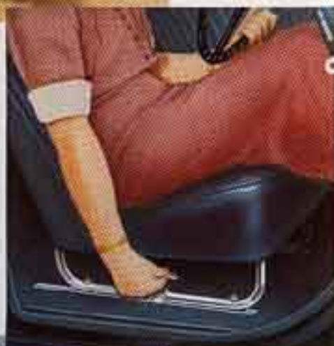
The driver's seat of the four-door saloon is instantly adjustable for position, while the passenger's seat can also be adjusted. On the two-door saloon and open models the front seats are of the tip-up adjustable type.
