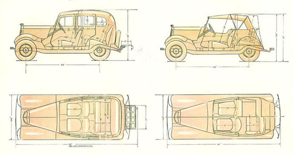
The front seats are provided with a range of adjustment of 3 inches and are shown midway in this range in the illustrations.
