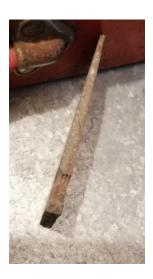
Series 1 & 2 Axle wedge on its edge The large photo below is from above
