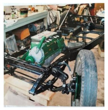
During the dismantling it was discovered some significant damage to chassis cross members, timber framing and panel repair. It dawned on me at this point that the damage and repair work undertaken (which included items such as headlight shells, parking light shells, radiator surrounds, running boards and guards) was most likely due to a "light rollover" my father once mentioned happened during the war years.
