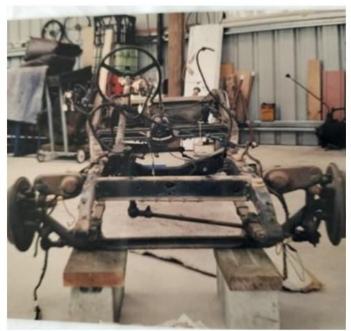
The chassis and all mechanicals were stripped, caustic cleaned, repaired, treated and painted with particular attention to preserving ALL original parts including fasteners for re-use.
