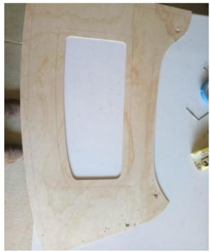
The second photo shows where I cut the shape of the outside and the pocket out with a jig saw and sanded the edges smooth. I marked out where all the locks and screws were to go and drilled them all. This is the inside of the driver's door. On the outside I glued 5mm foam then I glued the cream vinyl. The inside shows how I've cut and glued the vinyl to the ply.
