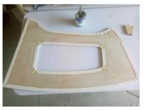
Photo no 3; here I've marked on the face of the vinyl at 50mm intervals on the bottom and 10, 32 and 10mm down from the top.
