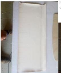
Photo no 4. I've crimped or gathered the bottom of the vinyl by folding over the vinyl at the 50 mm intervals.
