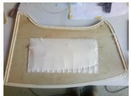
No 9. Here is the final part from the contorted mess before. All stapled onto the back of the door card ply. Nice and neat, now onto the next one.
