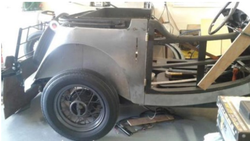
Figure 3: New panels made
