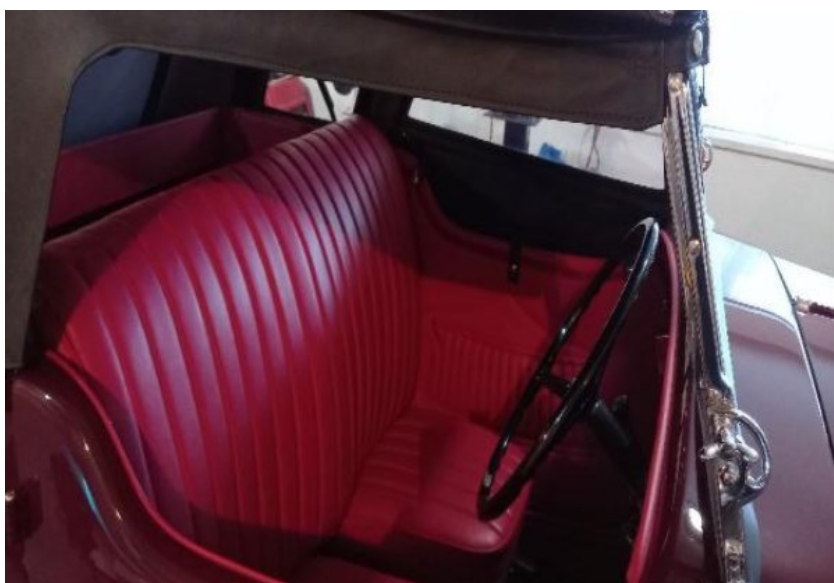
Figure 7: Upholstery fitted and completed
