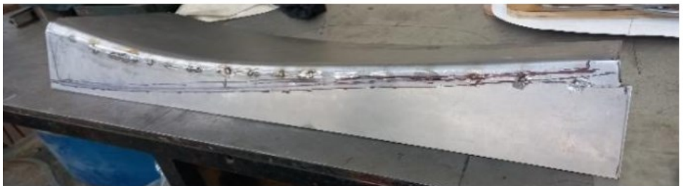
Figure 5: Running boards being made from template
