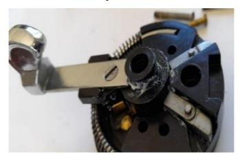
Assembled turn signal lever showing hinge levers, U-shaped brass contact and spring, washers set up for lever mechanism.
