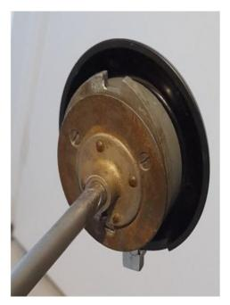
Switch with top of stator tube showing the three screws securing the base to the rest of the switch. The self-cancelling ring can be seen in the front of the Bakelite base.
