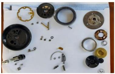
All the parts inside the switch. Top - Left to Right and around. Earth ring base with indicator contacts. Self-cancelling ring with felt pad to reduce rattles. Base plate at top of stator tube. Horn button parts. Sliding brass contact for left and right indicators, spring positions, hinge levers. Turn signal lever with roller and spring. Bakelite base that all the parts fit into.
