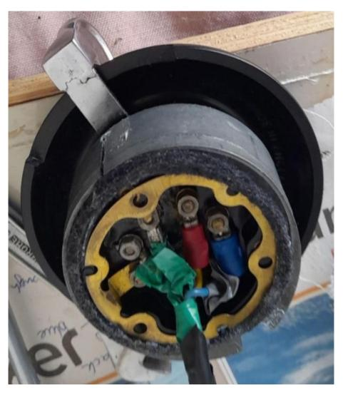
View of wiring and earth ring. Lower left is the earth ring and through screw screw/nut. Above that on the left is the left trafficator wire. Next on right is the power feed wire, next is the right trafficator (yellow/red) and blue cable is the horn wire and also the through screw/nut to hold the assembly together
