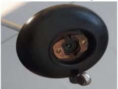
All components of the switch were then cleaned, given a slight smear of white lithium grease to provide lubrication for the turn signal lever, the roller and the two hinge levers and the Bakelite where those parts meet.
