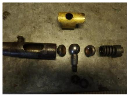
The drag link was disassembled, cleaned and put together with fresh grease.
