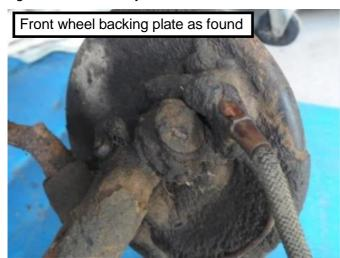
The brakes were disconnected, steering draglink removed, track rod disconnected, front shackle bolts knocked out and rear shackle pins removed. The assembly could now be lowered to the ground and spring U bolts removed.
