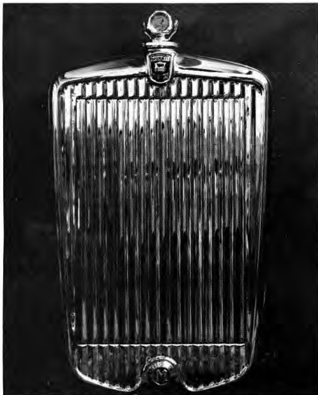
Morris Oxford 1932-33. The "M" cover over the starting handle hole was common in size and design for all the contemporary Morris models that had this fitment.
