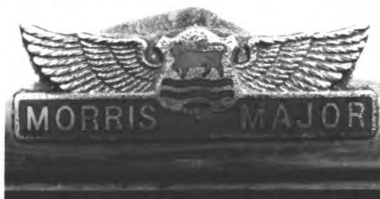
Morris Major 1931 (Chassis numbers MJ.101 to MJ.4125. From MJ.4126 the Major had a shield shape badge, part no. 55206). A similar badge to that above was used on the 1930-31 Oxford. Blue background to the lettering (Chassis LA101 to LA23746, Badge part no. 45152).
