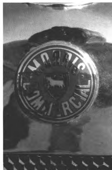
Type of badge fitted to vans chassis 30001 onward, Badge part number 16133. Probably 1924 to 1926.
