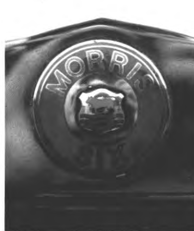
Morris Six, 1928 & 1929. Inner circle is plated with shield in bas-relief. Letters filled in green with a blue background.
