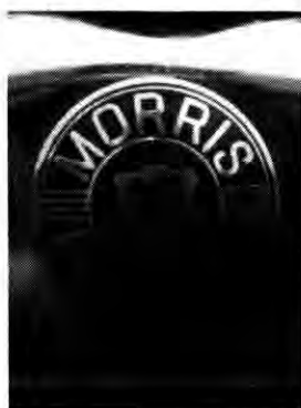
Minor type 5 cwt light vans 1930-34. Colour details as the 1929-31 Minor cars. (O.H.V. and early S.V. versions, Badge part number 17286. S.V. vans had a change in part number to 35846 in August 1932 and to part number 37519 in May 1933.
