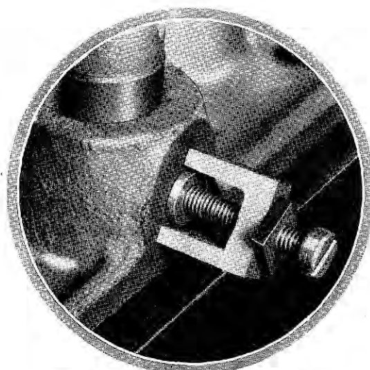
A simple extractor can be made to withdraw the distributor drive spindle dowel.
