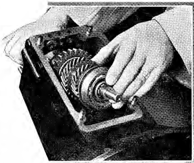
Showing the method whereby the sliding shaft assembly is removed.
