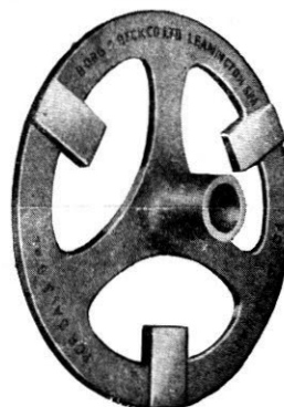
Fig. 8. Below.—The special Borg and Beck gauge plate necessary for setting the release levers.
