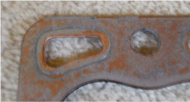
Gasket with all coolant holes swaged
