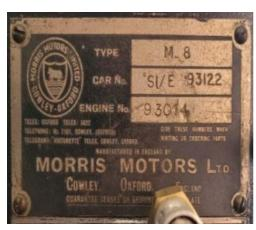
The VIN Plate is the first reference and then you can check if your Chassis and Engine Numbers match.
