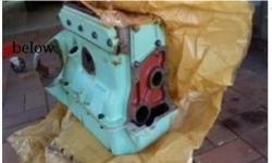
able to see that the block is a late MM with a water jacket just the top of the block, the hole for the oil filler next to the starter and a boss for an external oil filter. On the front of the motor is provision for a water pump, blanked off, a dip stick hole (a
