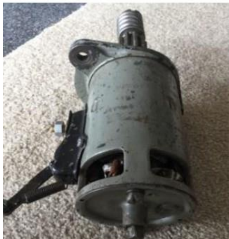
The fitted starter motor with integral manual switch and 3-hole mounting flange.
