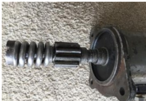
The fitted starter motor with integral manual switch and 3-hole mounting flange.
