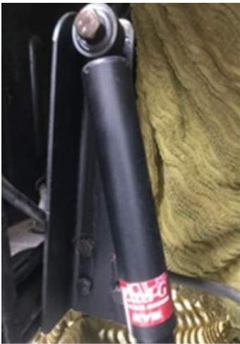
(view from front) LHS shock and bracket fitted, showing top attachment to the new bracket and bottom attached to the axle mount.
