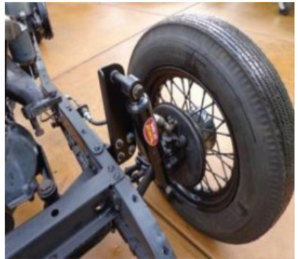
Earlier conversion kit for front shock absorbers (internet source)
