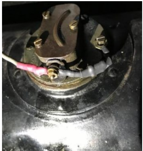
Sender unit reinstalled with shunt resistors
