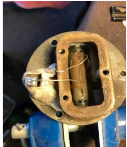
New soldered connection to the resistance element at the bottom
