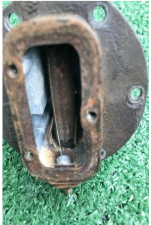
Sender unit with cap removed
