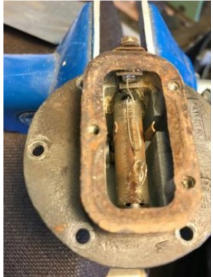
New wire terminated and old connection left loose
