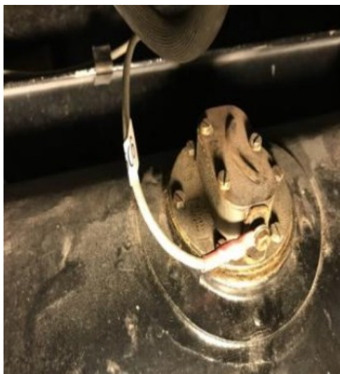
The sender unit with connection to the gauge.
