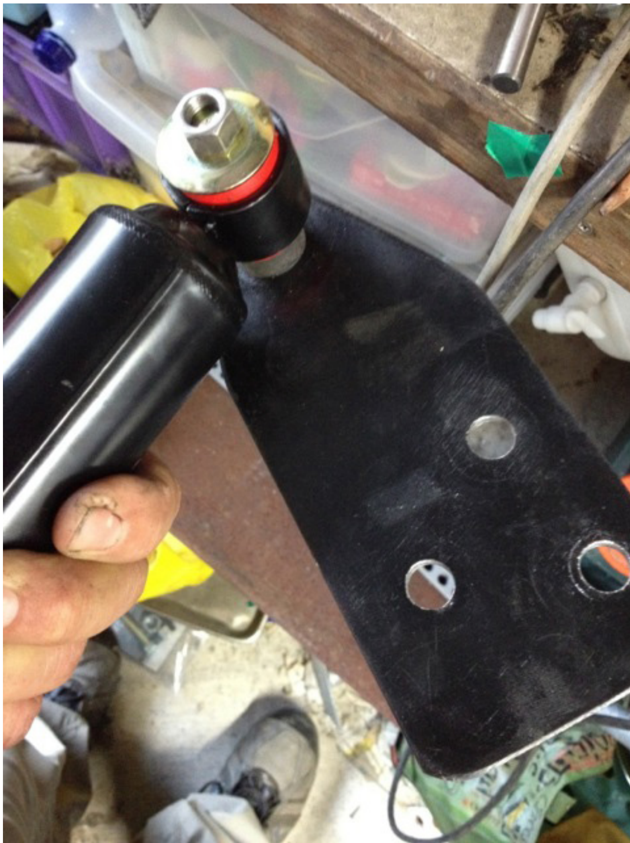
Shock bolted to plate before bolting to chassis
